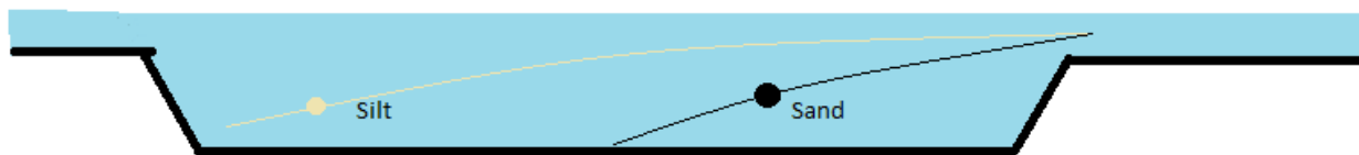
Figure 2 Schematic showing settling dynamics of sand and silt particles in a flowing sediment basin
